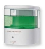
Unit Size: L110\*W128\*H132mm Volume: 600ml Working Voltage: DC6V Working Current: 120mA Standby Current: 50uA Sensing Distance: 0-8cm Power Supply: 4 "AA" batteries Packing: 30pcs/ctn Carton Size: 630\*423\*308mm
