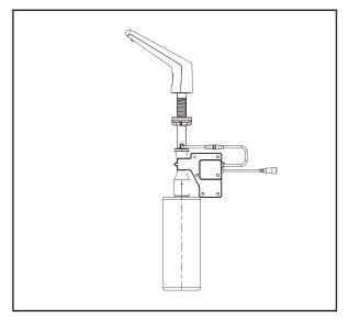
Unit Size: L141\*W40\*H130mm Volume: 1000ml Working Voltage: AC100-240V 50/60Hz Sensing Distance(adjustable): 2-14cm Liquid Duration Time(adjustable): 0.5-3.5s Liquid Amount(adjustable): 1-4ml
